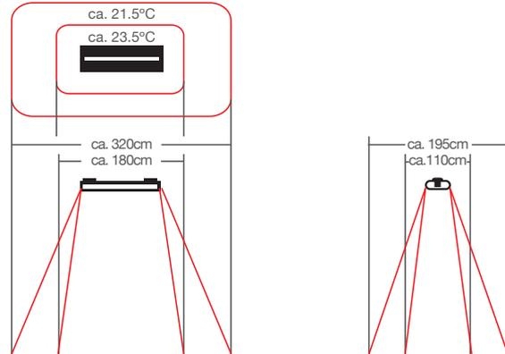
Temperatures shown are in a cold, windless space with an ambient temperature of 16.5°C, with the unit mounted at 2.5 metres.
